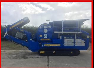
An impressive 900 x 450 Jaw Crusher. Small & Compact, with relatively low weight - No compromising on the strength and overall performance for this size of crusher. The new grizzly feeder, optimises crusher throughput. The power unit and hydraulic functions remain simple, allowing all end users to easily operate, and carry out basic maintenance as and when required.
