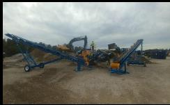
OPTIONAL EQUIPMENT: THREE (3) 40' RADIAL STACKING CONVEYORS
